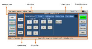
Click the Configure button from the Selection pane, or select Tests > Configure from the menu bar to change the configuration settings.
